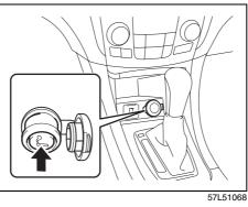
The cigarette lighter will work when you press the engine switch to change the ignition mode to "ACC" or "ON".
